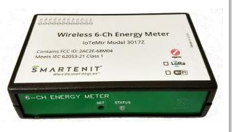
The IoTeMtr can be configured for various current levels as its six current sampling channels are set up for current transformers (CTs) with a 333mV full range output. Smartenit offers a wide range of CTs to satisfy most needs.
