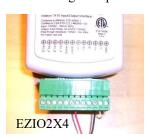
for the EZIO8T. It also possible to use one of the opto-isolated inputs. In this case, the red wire of the sensor is connected to the +V source, and the black wire to the (+) side of the selected input. The (-) side of the input is connected to ground (GND.) Thus connected, the sensor asserts the input ON when it trips. If the
