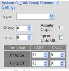
The analog and 1-Wire sensor can be "digitized" to provide the Off to On and On to Off transitions at preset points or alarms.
